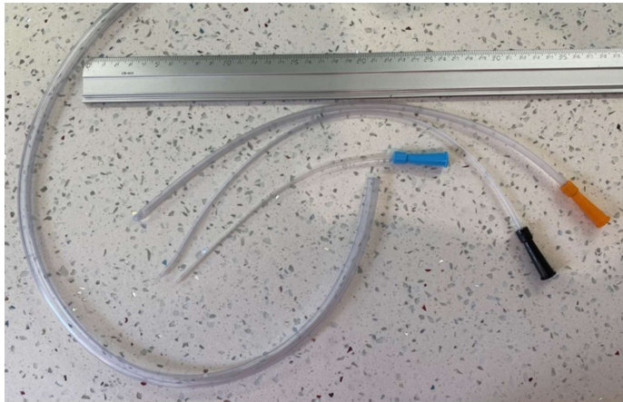
Figure 4 – Cannulas A (orange) and C (blue) and 6mm tubing used in tests
